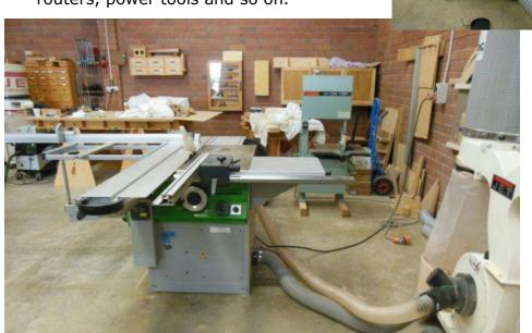
The task of dust abatement was shouldered by two Jet cartridge extractors – one double and one single cartridge unit – plus two Festo vacuums.
